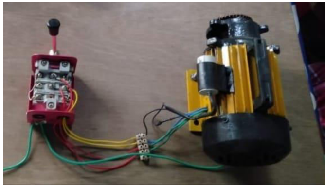
Fig.1 wiring diagram of drum switch and induction motor
